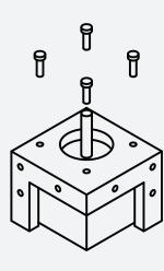
Insert the Stepper Motor into the base of the **Right Front Motor Mount**
